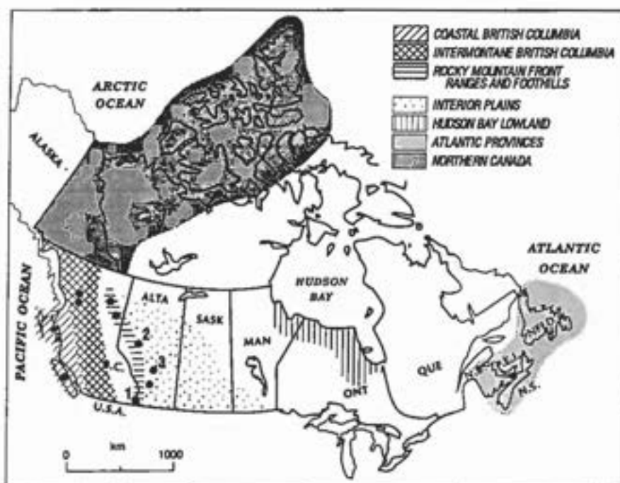
Fig. 1: Distribution of coal-bearing basins in Canada (Smith, 1989) and areas (o) currently being evaluated for coalbed methane potential. Locations discussed in this paper: 1 = Front Ranges, British Columbia; 2 = Foothills and Plains, west-central Alberta; 3 = Plains, Alberta.
